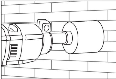
1. To minimise cracking, drill a pilot hole and then core drill from both sides into the cavity.
