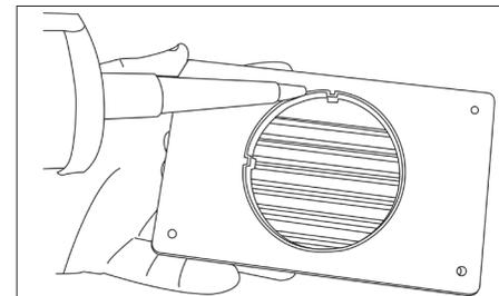
8. Insert the louvre grille and backplate assembly into the exterior end of the tube.
