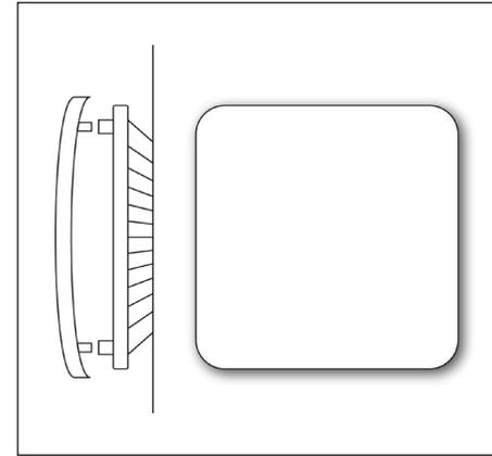
Rytons fixed open LookRyt panel is for the provision of combustion air to boilers, stoves and fires.
