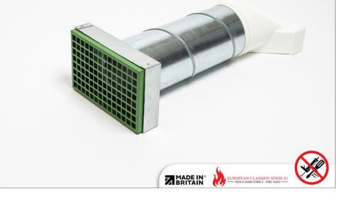
Rytons A1® Fire-rated Ducting Kit 125mm Dia. with Square Holed Double Air Brick Custom RAL colour air brick in matt, semi-gloss or gloss finish achieving Class A2-s1, d0 RAL6010 (Grass green) matt finish pictured Connector for 125mm dia. ducting Registered Design 6109953 Patent Pending Product Code: A1DK125SQD
