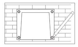
**Cowled models:** Screw the cowl to the brickwork through the preformed holes in the flange around the cowl. Fittings not supplied.
