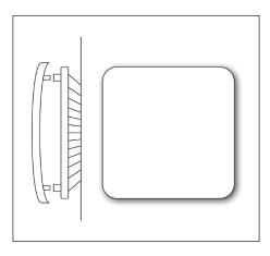
Rytons fixed open LookRyt panel is for the provision of combustion air to boilers, stoves and fires.
