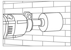
1. To minimise cracking, drill a pilot hole and then core drill from both sides into the cavity.
