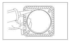
DO NOT clip the internal LookRyt panel to the backplate until the backplate is fixed to the wall.
