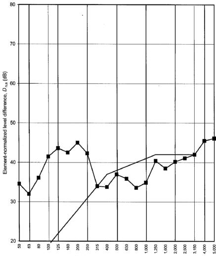
x Adjusted for flanking transmission
